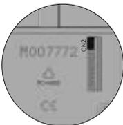
The end of line jumper is placed on the video module of the CN2 connector, that is located on the back side of the monitor.
