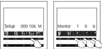
To select the monitor option Mon press the indicated menu push button, then change the three digits with the option ↑ until you get the desired monitor address.
