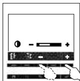
To select the contrast option press ● the push button of the menu as indicated, then adjust to the desired value.
