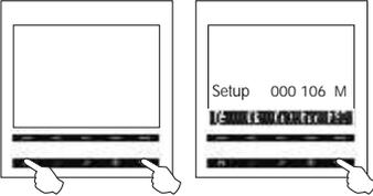
With the door release push button pressed switch on the monitor.
