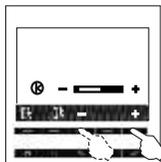
To select the colour option press the ⊕ push button of the menu as indicated, then adjust to the desired value.
