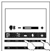
To select the audio volume option press the 🔊 push button of the menu as indicated, then adjust to the desired value.
