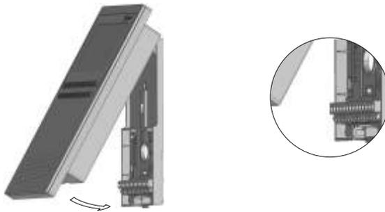
To disassemble the monitor from the connector, use a plain screwdriver to release the attachment clip. Pull the monitor towards you to remove it from the connection block taking special care that it does not fall.
