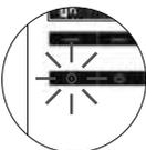
Press the door panel push button that will call to this monitor. At this moment the door panel will reproduce a sound and the monitor led will blink.
