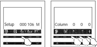
To select the column option Col press the indicated menu push button, then change the three digits with the option ↑ until you get the desired column number.
