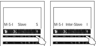
To configure the monitor as slave or inter-slave, select the MSI option pressing the indicated menu push button, then press repeatedly the ↑ option until the desired option appears.
