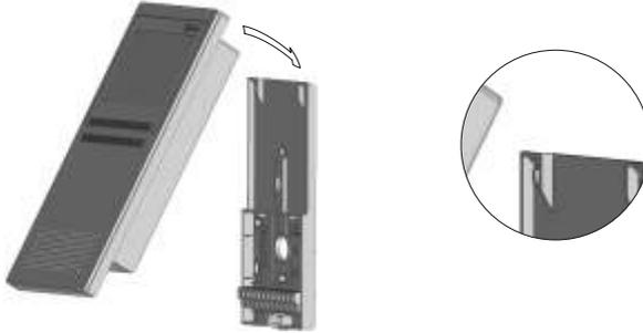
Lock out the monitor pressing its lower side till the attachment clip locks the monitor firmly.
