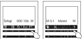
To configure the monitor as master, select the MSI option pressing the indicated menu push button, then press repeatedly the ↑ option until the master option appears.
