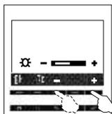
To select the brightness option press the ☒ push button of the menu as indicated, then adjust to the desired value.
