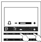
To select the call reception option press the 📞 push button of the menu as indicated, then adjust to the desired value.
