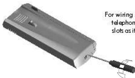
For wiring and fixing purposes, it is necessary to open the telephone. Lever slightly with a plain screwdriver into the slots as is shown in the picture.
