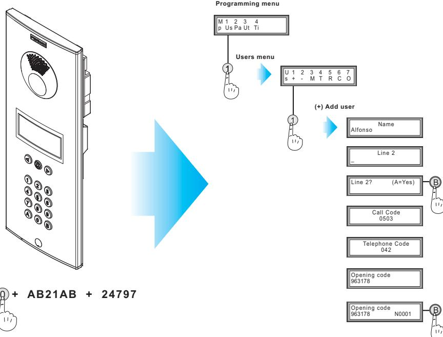
Programming sequence of call code must be done as described in the diagram and only can be made in panels with Display. **Detailed information in this manual.**
